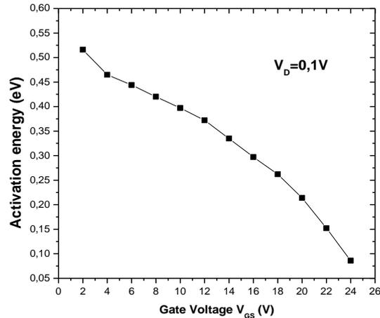
Fig.4. The evaluated activation energy versus the gate voltage.
