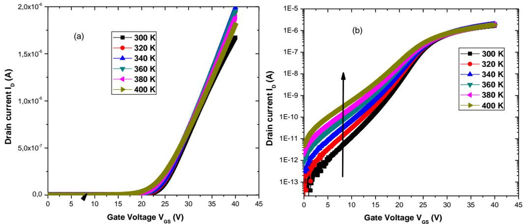
Fig.2. The simulated transfer characteristics  $I_D = f(V_{GS})$  of the TFT for different temperatures ranging from 300 to 400 K on linear (a) and logarithmic (b) scales.
