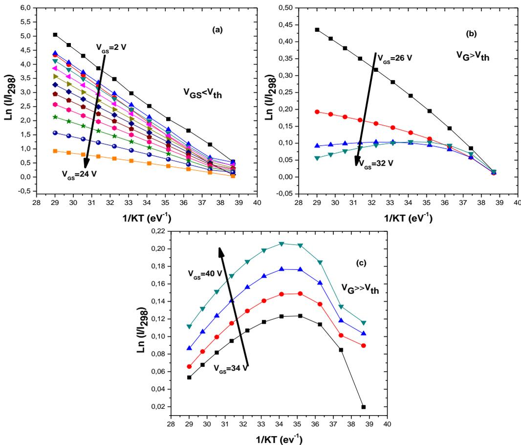
Fig.3. The Arrhenius plot of the normalized current  $I/I_{298}$ . (a) in the sub-threshold voltage, (b) just on the onset of the threshold voltage and (c) well beyond threshold voltage.  $I_{298}$  is the current at 298 K.
