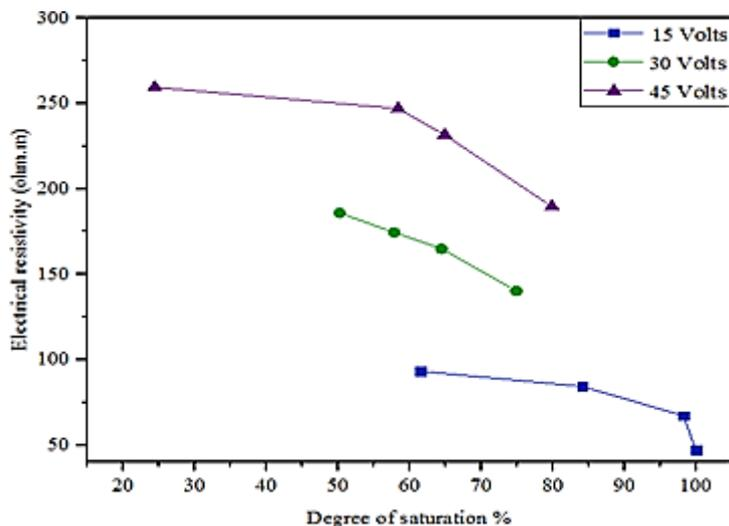
Fig.4. Effect of degree of saturation on electrical resistivity at 15, 30 and 45 volts.
