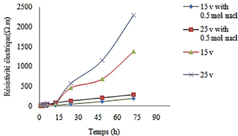
Fig.6. Variation of the electrical resistivity as a function of time for 15 and 25 volts.
