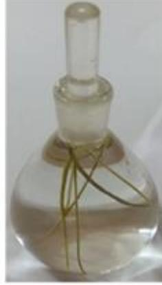
Fig. 3. The pycnometer used in measurement.
