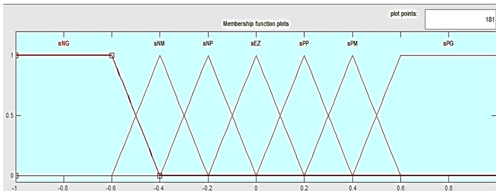
Fig. 11. Output variable membership function.
