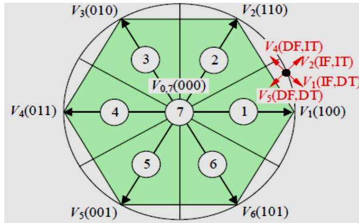
Fig. 2. Different vectors of stator voltages provided by a two levels inverter, (100): (1: inverter switch is ON, 0: for OFF) I(D) F: increase (decrease) of flux magnitude, I(D) T: increase (decrease) of torque.
