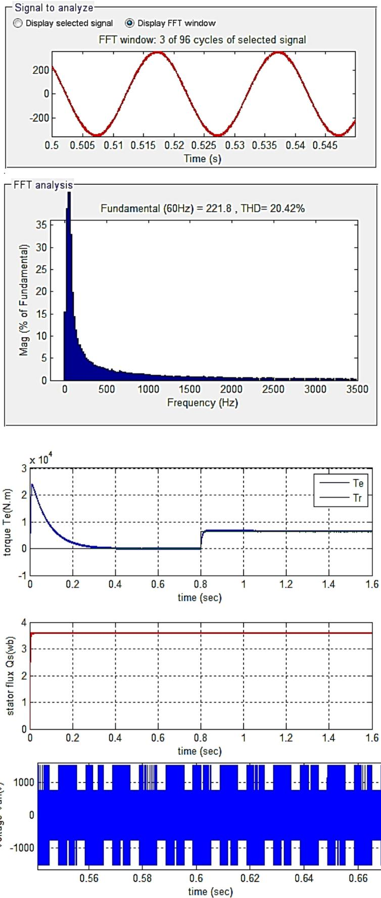
Fig. 12. Performances of classical DTC for IM.
