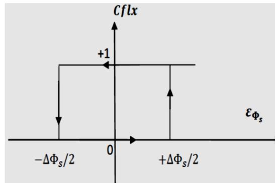
Fig. 4. Flux hysteresis comparator.
