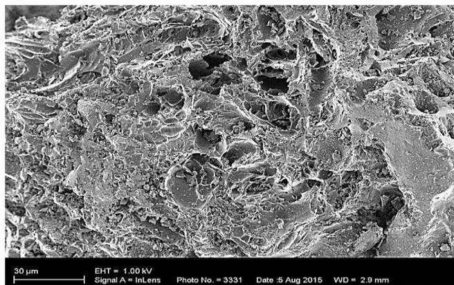
Fig. 1. High magnification FESEM micrograph of activated carbon.
