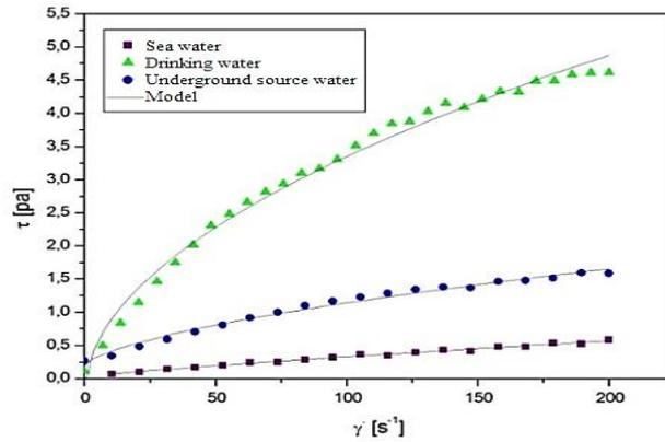
Fig.7. Rheogram for three water qualities emulsions with a concentration of 30% oil (type e) and 70% of water.
