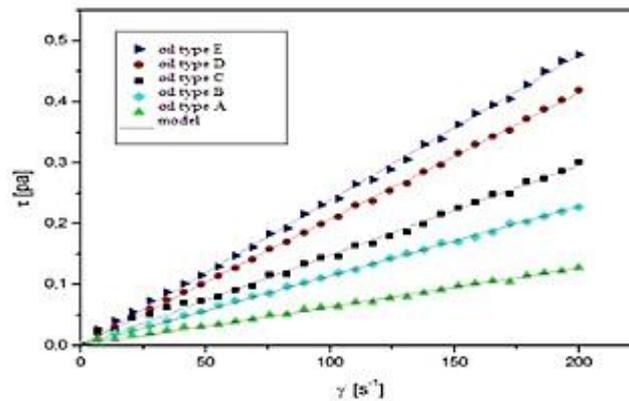
Fig.2. Flow curve for crude oil at ambient temperature of 23°C.
