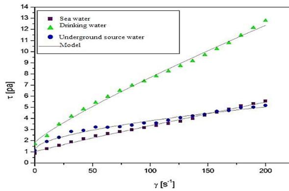
Fig.5. Rheogram for three water qualities emulsions with a concentration of 30% oil (type c) and 70% of water.
