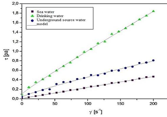
Fig.4. Rheogram for three water qualities emulsions with a concentration of 30% oil (type b) and 70% of water.
