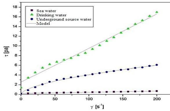
Fig.6. Rheogram for three water qualities emulsions with a concentration of 30% oil (type d) and 70% of water.
