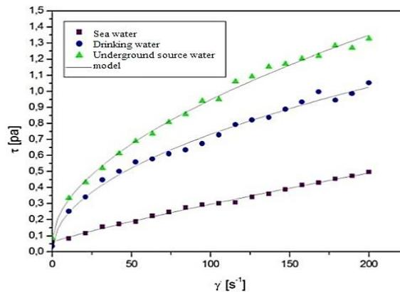
Fig.3. Rheogram for three water qualities emulsions with a concentration of 30% oil (type a) and 70% of water.
