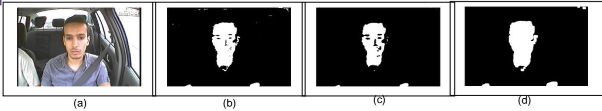
Fig 2. Morphological operations on the mask of skin color, (a) Image original, (b) Mask M of skin color detection, (c) Erosion, (d) Dilation.
