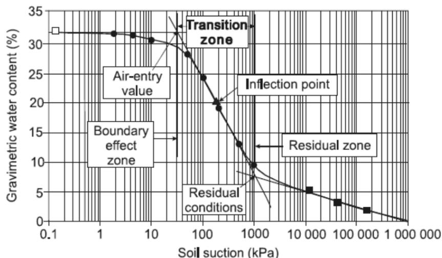
Fig.1. Typical SWCC and Identifiable zones (Vanapalli et al., 1999).
