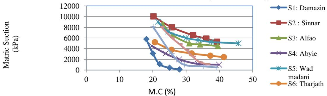
Fig. 2. SWCC for tested soils from different parts of Sudan.
