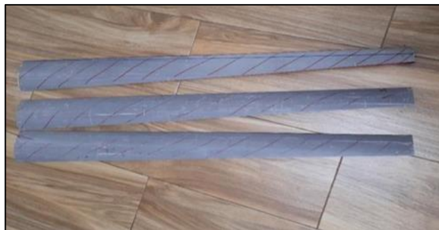
Fig.3. Three blades obtained from a single 200 mm diameter PVC tube after cutting.
