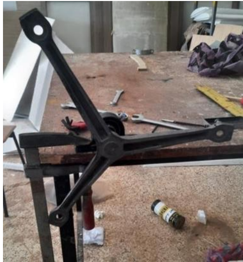
Fig.4. Metal shaft recovered from a washing machine used as the main hub axis for the prototype.
