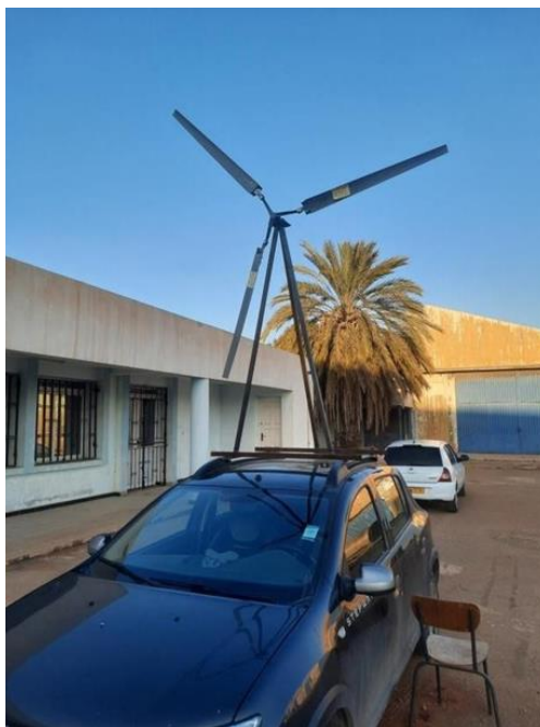
Fig.5. Mobile testing configuration: wind turbine mounted on the top of a moving car to simulate real airflow conditions.
