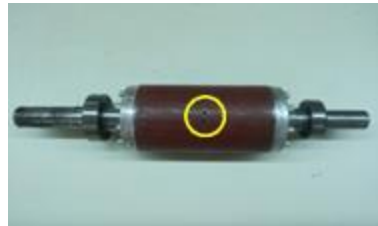
Fig. 5. Faulty rotor used with two broken bars.
